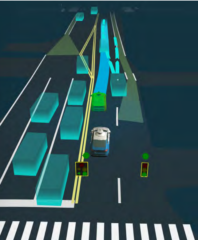
Playforward In this simulation, we look at what our test vehicle was projected to have done, as noted by the green vehicle, if the Test Specialist had not disengaged the self-driving system.
